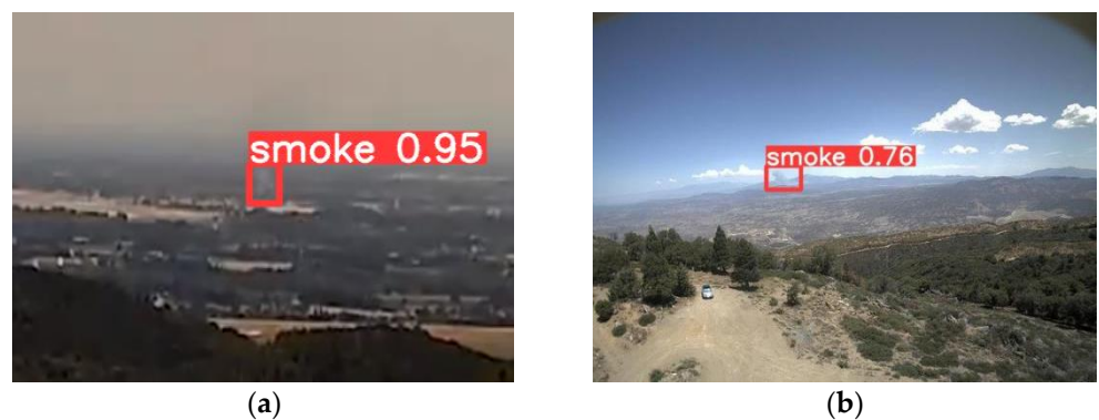
Figure 13. Recognition results of small smoke and smoke with interference containing something similar to smoke in images: (a) Small smoke; (b) Smoke with interference containing something similar to smoke in images.
