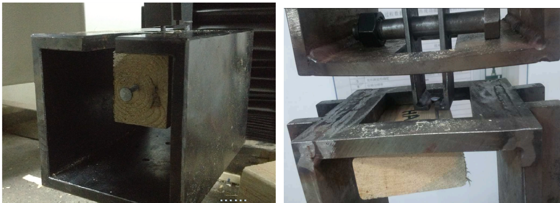
Fig. 3. Nail holding power test
